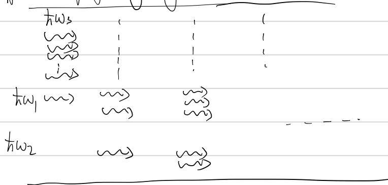
So Difference frequency generation is also called parametric amplifier. Why "parametric"? The state of the material is unchanged.
