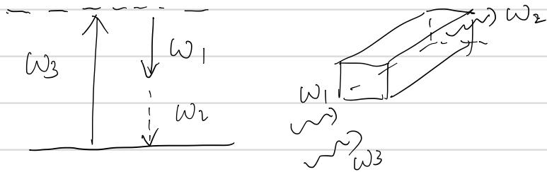
Input  $\omega_1$  and  $\omega_3$ , get difference frequency at  $\omega_2 = \omega_3 - \omega_1$ ,
