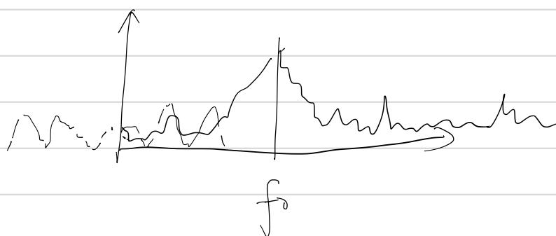
If the modulation rate is higher than carrier frequency, you will create base-band folding, and destroy the information.
